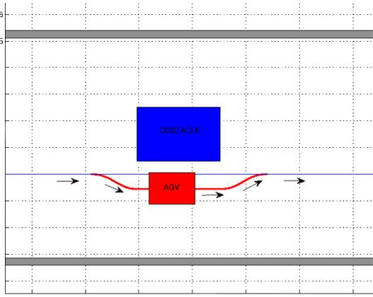
Fig. 8: Overtaking of an obstacle which is not on the roadmap, but too close to it
