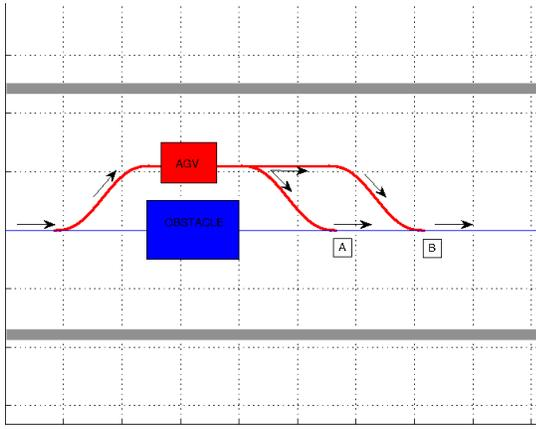
Fig. 6: Return on the roadmap: the overtaking can end in different parts of the roadmap depending on the actual space. Points A and B are two possible points of attachment to the roadmap.
