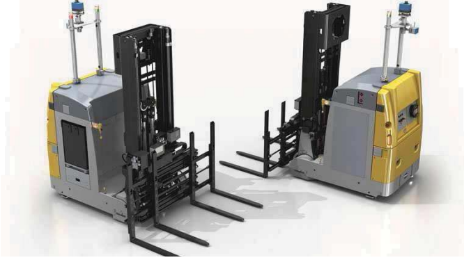
Fig. 2. AGV with forks for object transportation
