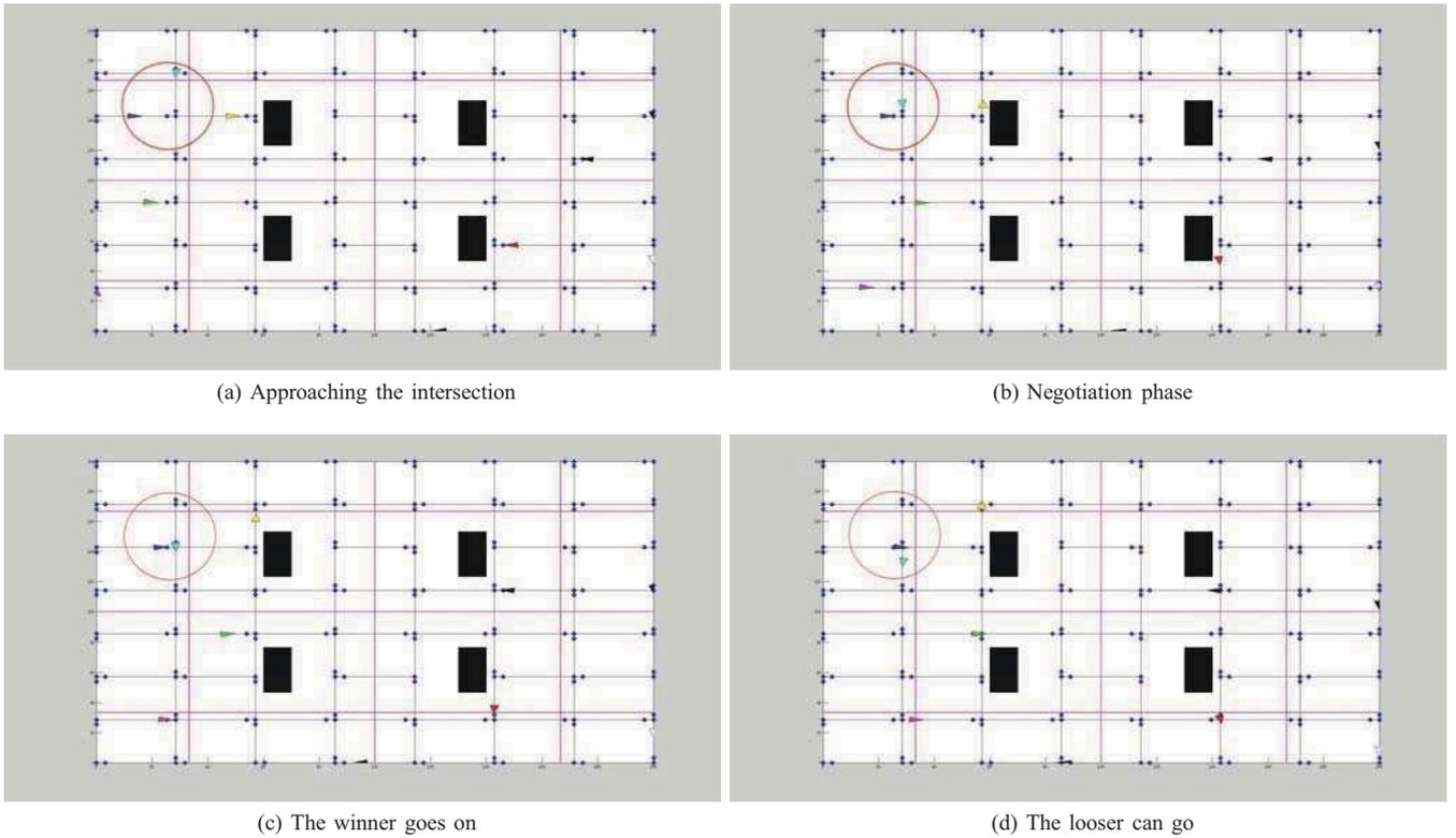
Fig. 5: The screen-shots show the coordination at intersection. In these pictures, the red lines are the segment's borders and the dots are the nodes of the route map
