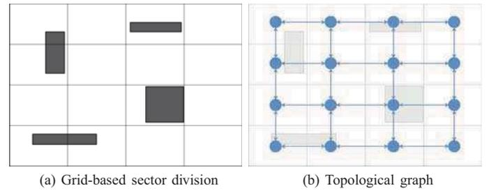
Fig. 1: The topological sector division: in 1a the geometric map is divided into regular sectors; in 1b the graph representation generated by the sector division is shown
