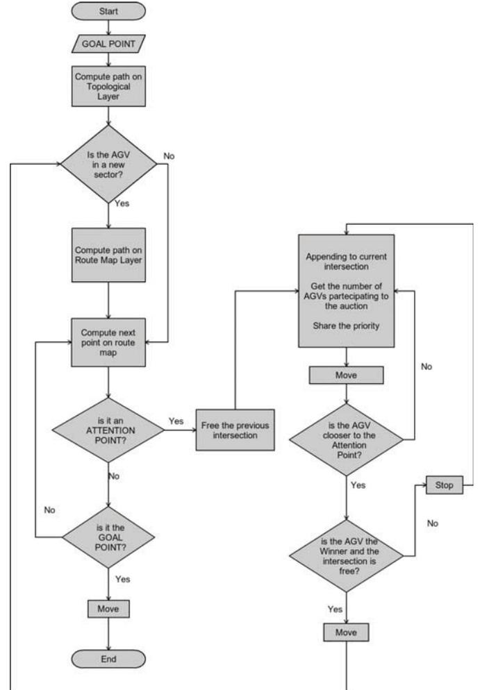
Fig. 4: Flowchart diagram of the path planning and coordination procedures.
