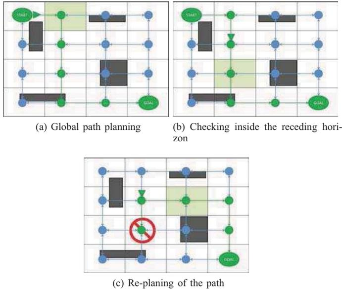
Fig. 2: The path planning on the topological layer: in 2a the path is searched by means the D\* algorithm; in 2b the AGV moves along its path and checks the next sectors; in 2c a re-planning of the path is needed due to the new condition of the next sector
