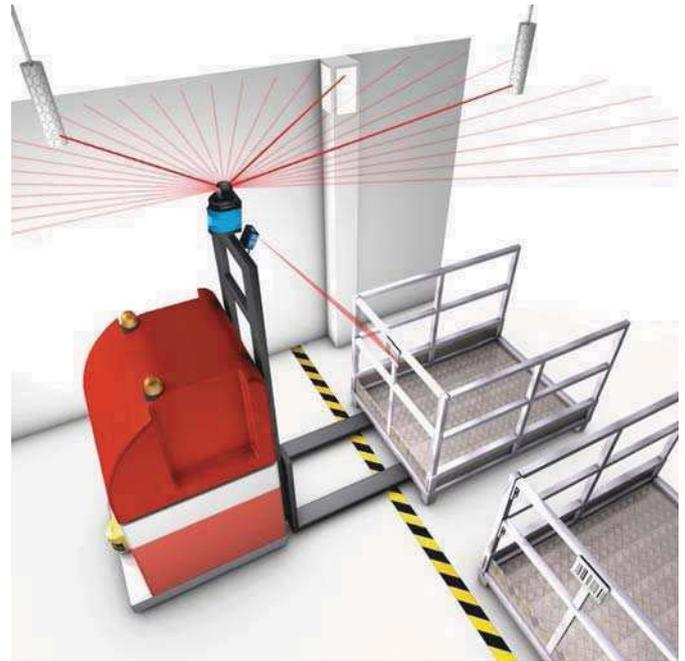
Fig. 1. Reflector-based localization like performed by the SICK NAV 350 Laserscanner is currently state of the art in AGV localization in industrial environments. [1]
