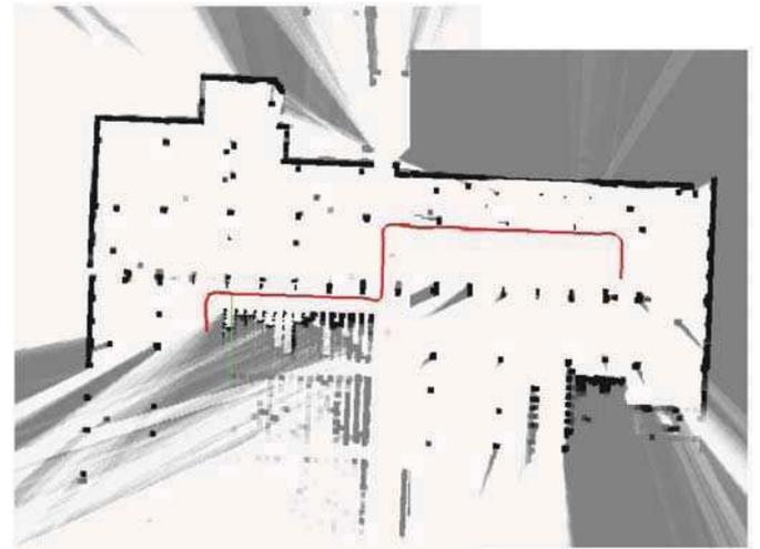
Fig. 9. The trajectory used for evaluation plotted in the grid map of a part of the warehouse of Casbega in Madrid, Spain.
