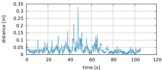
Fig. 11. The position difference between the contour-based and the reflector-based self-localization.
