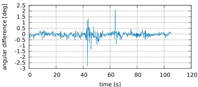
Fig. 12. The angular difference between the contour-based and the reflector-based self-localization.
