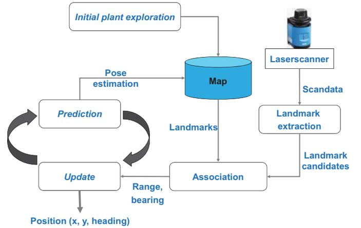
Fig. 7. Architecture of contour-based self-localization system.
