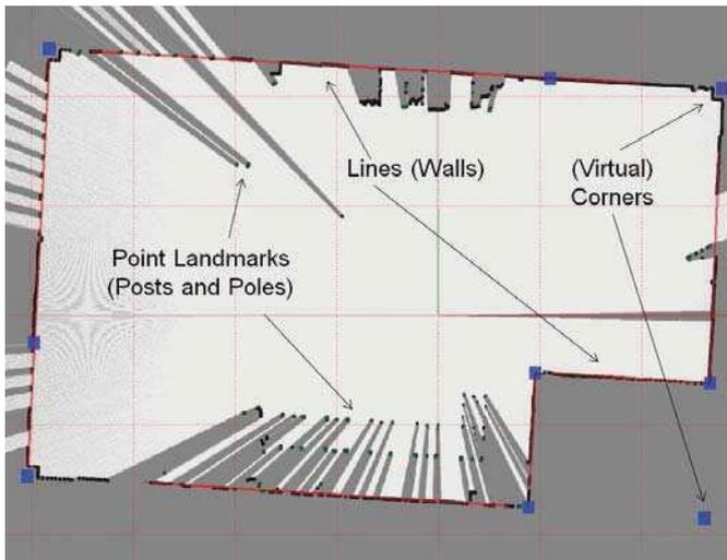
Fig. 8. Extraction of various different natural landmarks.
