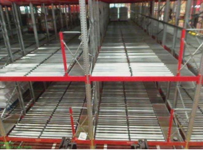
Fig. 5. A gravity rack in the Casbega warehouse in Madrid, Spain.
