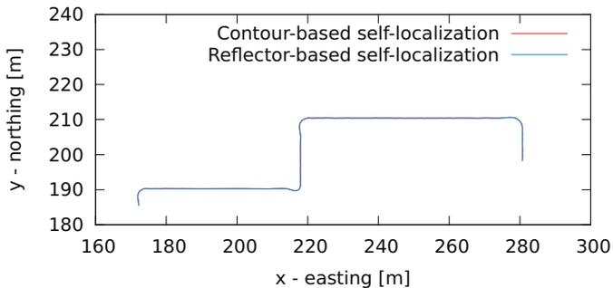
Fig. 10. Comparison of the trajectory of the contour-based self-localization with the reflector-based self-localization done by the SICK NAV 350. Both trajectories align at this resolution, the difference is plotted in Fig. 11 and 12.
