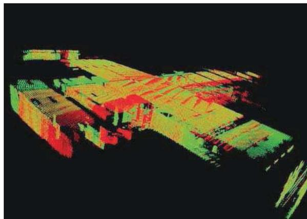
Figure 9. Result for a successful scan registration of two scans (in red resp. green) of the 3D Laserscanner at two positions. Distance between positions was approx. 2 m. Consistency is observable, e.g. at the left side where one part of the warehouse wall was covered at one scanner position and the other part from the other position. Together they result in a straight wall with some overlap that is colored in yellow.
