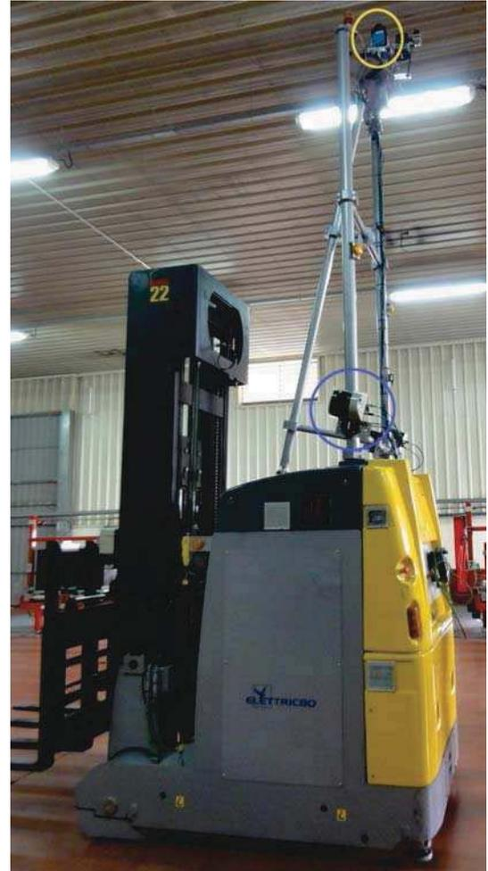
Figure 3. The mapping AGV equipped with multiple Laserscanners. On top blue coated NAV350 – encircled in yellow – with 360° horizontal field of view, in the middle attached gray coated LMS500 – encircled in blue – to scan the environment perpendicular to the direction of the AGV heading.
