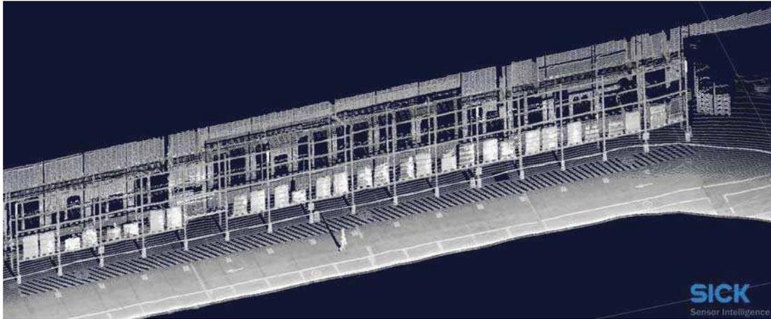
Figure 4. The measurement data recorded by the mapping AGV with support of the current NAV build-in reflector localization.
