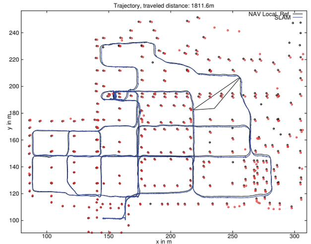
Figure 6. Result map and trajectory. Black circles are positions of reflectors in the reference map, red circles are the map entries generated by the employed Feature SLAM
