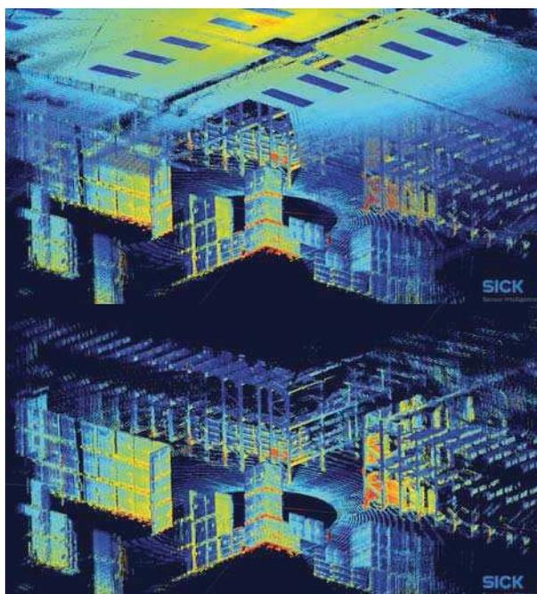
Figure 8. Measurement result for 3D Laserscanner at one position, note the repeating structures of the racks (back) and pallet blocks (front). Upper image shows the full scan, while in the lower image the point cloud is clipped at a height of approx. 5 m in order to have a complete view on the racks.
