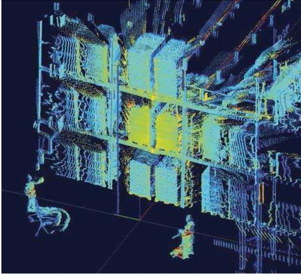
Figure 5. Top-down scan swath of a gravity rack using a SICK LMS100. False color indicate reflectivity (RSSI) - blue represents low RSSI, red high RSSI values.
