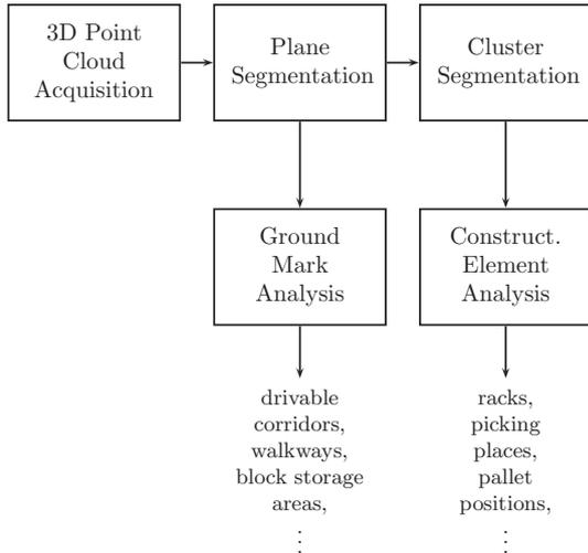
Figure 1. Warehouse element recognition pipeline consisting of multiple segmentation steps and feature extraction.
