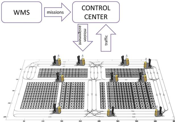
Fig. 2. Multi-vehicle system in industrial applications: architecture
