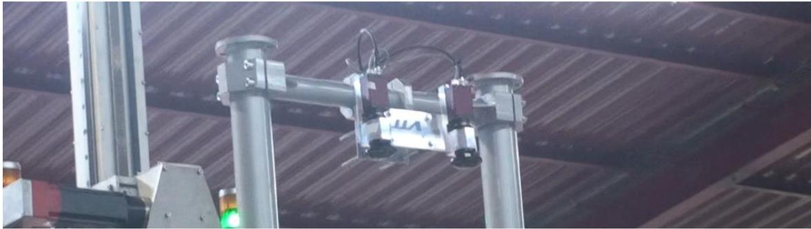
**Figure 2: Mounted omnidirectional stereo camera sensor**
