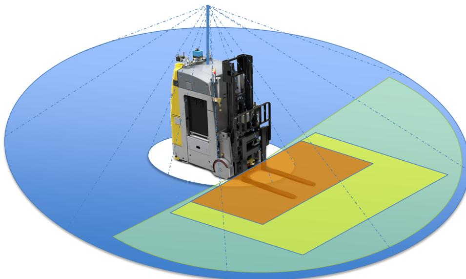
A low-level fusion of the four safety laser scanners provides a very consistent and precise 2D observation all around the AGV. In addition the background elimination removes all measurements of static objects registered initially in the 3D semantic map, which enables a very efficient and reliable object tracking and classification. The objects are correctly tracked and classified and the required accuracies are achieved on the test data sets.
