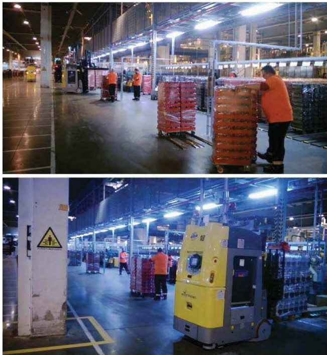
Fig. 3: Human operators sharing the environment with AGVs
